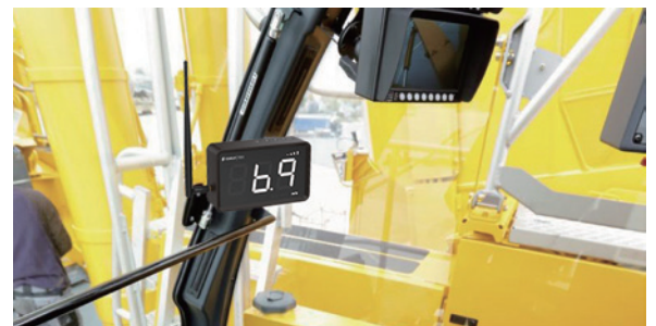
Large wind speed display for crane operators
