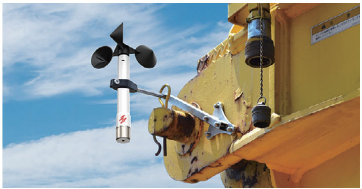
Magnetic self-leveling mounting bracket for easy installation
